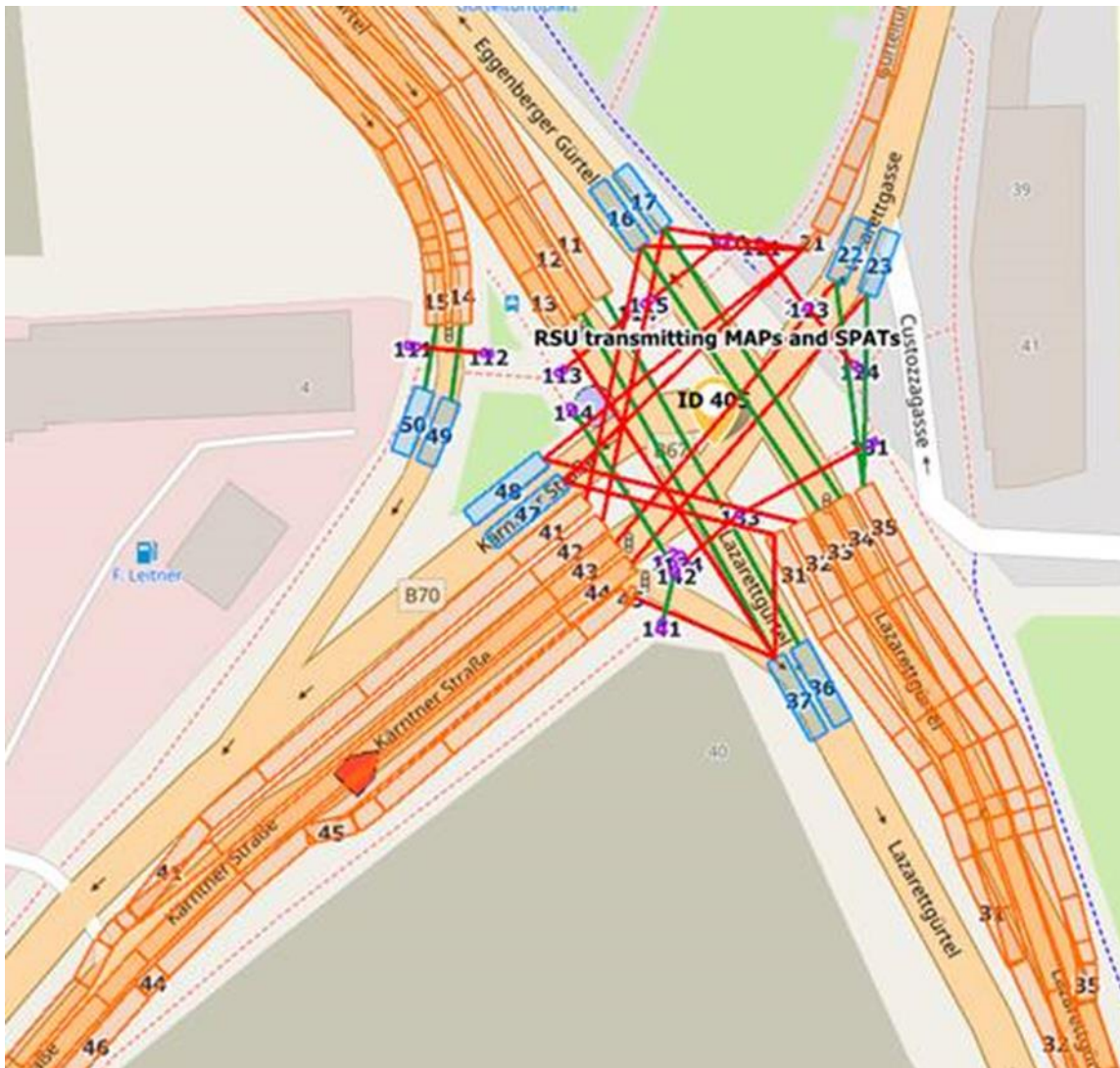
Picture 3: SPAT/MAP Message from the City of Graz/ Austria (Intersection: Lazarettgürtel / Kärntnerstraße)
