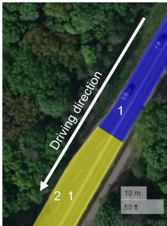
Figure 38: ADASIS-road segments for the scenario in clause 3.4 with the expected ETSI LanePositions. (Source: created using https://geojson.io © Mapbox (see: https://www.mapbox.com/about/maps/ ) © Maxar (see: https://www.maxar.com/ ))
