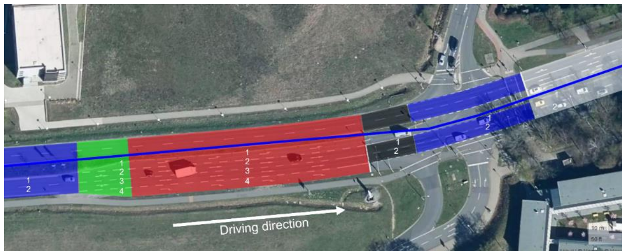
Figure 44: ADASIS-road segments for the scenario in clause 3.7 with the expected ETSI LanePositions for vehicles crossing the intersection straight. The solid line across the intersection is the more general path to follow. (Source: created using https://geojson.io © Mapbox (see: https://www.mapbox.com/about/maps/ ) © Maxar (see: https://www.maxar.com/ ))
