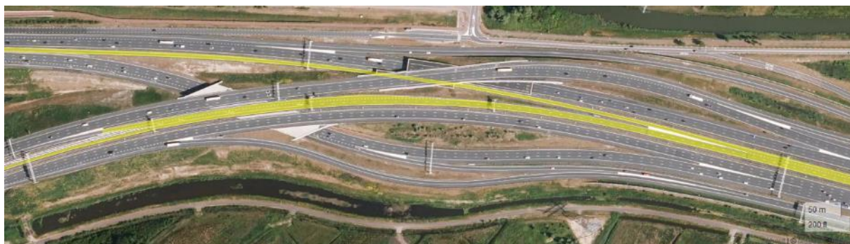
Figure 8: The revokable lanes of the motorway junction highlighted in yellow. (Source: created using https://geojson.io © Mapbox (see: https://www.mapbox.com/about/maps/ ) © Maxar (see: https://www.maxar.com/ ))
