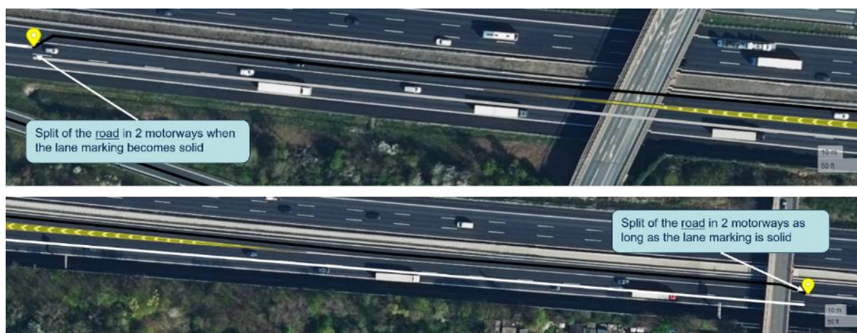
Figure 19: Scenario in clause 3.2 with yellow markers for the start and end points of road links and the different road links in between in white and black. The restricted area between the carriageways is highlighted in yellow. (Source: created using https://geojson.io © Mapbox (see: https://www.mapbox.com/about/maps/ ) © Maxar (see: https://www.maxar.com/ ))
