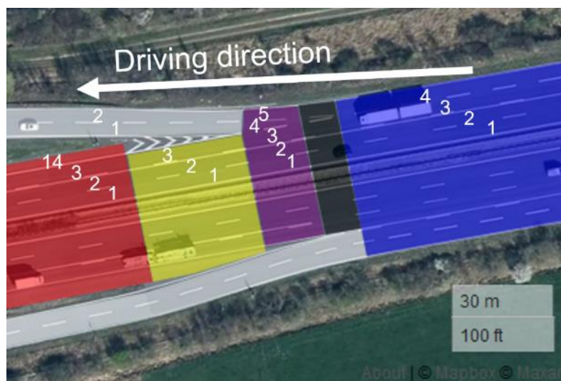
Figure 25: ADASIS-road segments for the scenario in clause 3.1 (where the second exit lane starts) with the expected ETSI LanePositions. The purple and grey segment use the same lane numbering, but it is not shown for the grey segment due to readability. (Source: created using https://geojson.io © Mapbox (see: https://www.mapbox.com/about/maps/ ) © Maxar (see: https://www.maxar.com/ ))
