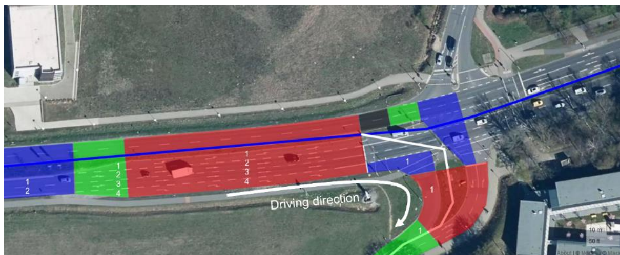
Figure 45: ADASIS-road segments for the scenario in clause 3.7 with the expected ETSI LanePositions for vehicles turning right. The solid line white line diverging from the blue one is the more general path to follow. (Source: created using https://geojson.io © Mapbox (see: https://www.mapbox.com/about/maps/ ) © Maxar (see: https://www.maxar.com/ ))
