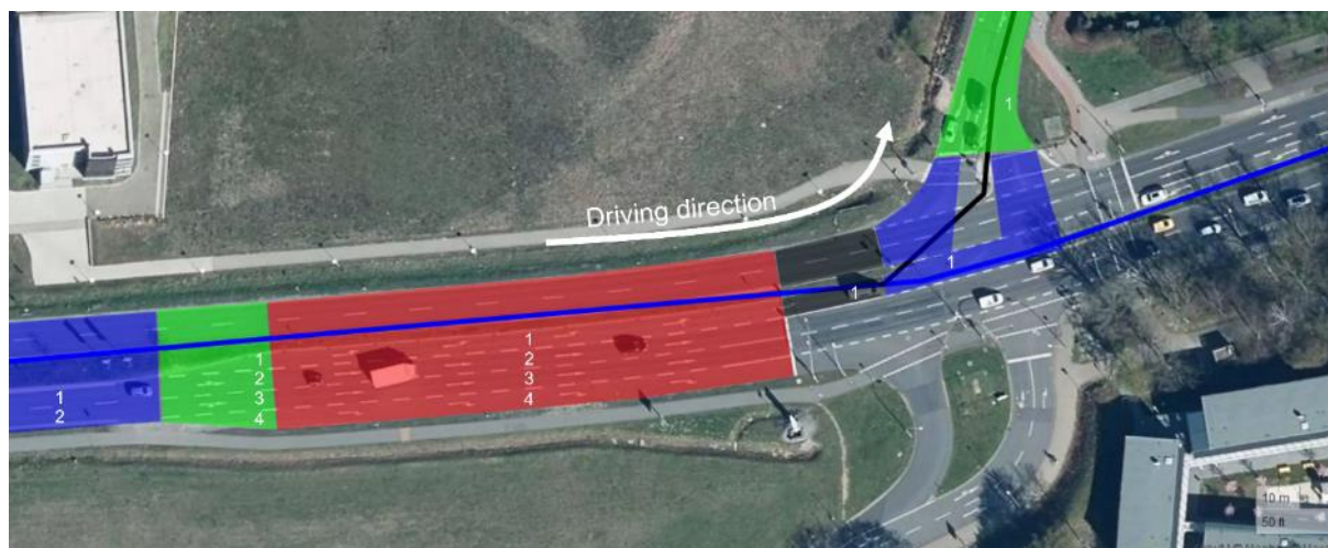
Figure 46: ADASIS-road segments for the scenario in clause 3.7 with the expected ETSI LanePositions for vehicles turning left. The solid line white line diverging from the blue one is the more general path to follow. (Source: created using https://geojson.io © Mapbox (see: https://www.mapbox.com/about/maps/ ) © Maxar (see: https://www.maxar.com/ ))
