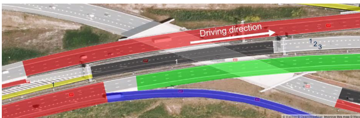
Figure 36: ADASIS-road segments for the central crossing of scenario in clause 3.3 (where the motorways crosses each other) with the expected ETSI LanePositions for the opposite direction. (Source: created using https://geojson.io © Mapbox (see: https://www.mapbox.com/about/maps/ ) © Maxar (see: https://www.maxar.com/ ))
