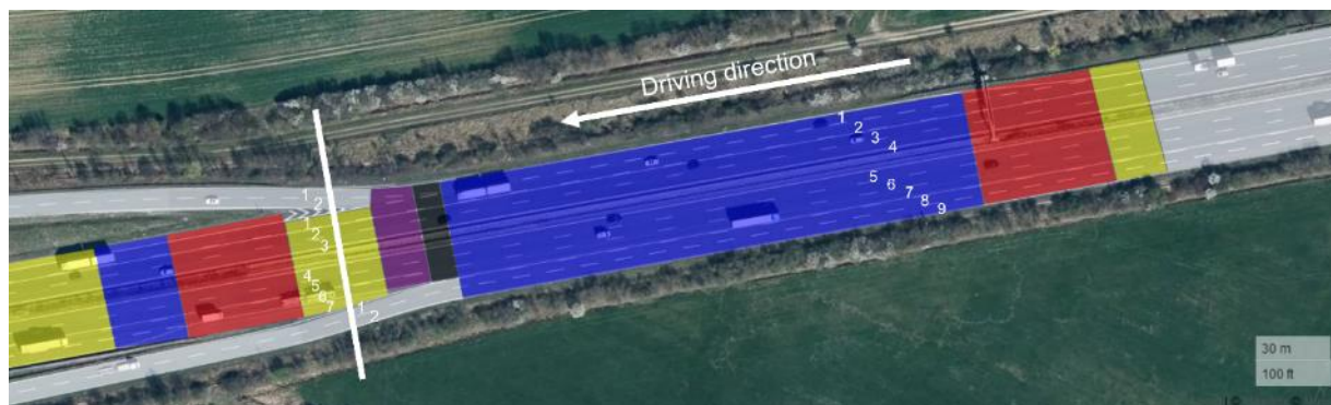
Figure 22: The solid white line represents the point for the transversal section of the entire road. The ADASIS lane numbers for the 3 segments at this transversal section are added. (Source: created using https://geojson.io © Mapbox (see: https://www.mapbox.com/about/maps/ ) © Maxar (see: https://www.maxar.com/ ))
