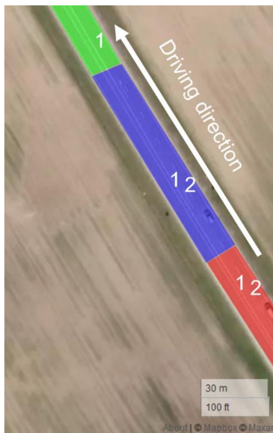
Figure 39: ADASIS-road segments for the scenario in clause 3.5 with the expected ETSI LanePositions. (Source: created using https://geojson.io © Mapbox (see: https://www.mapbox.com/about/maps/ ) © Maxar (see: https://www.maxar.com/ ))
