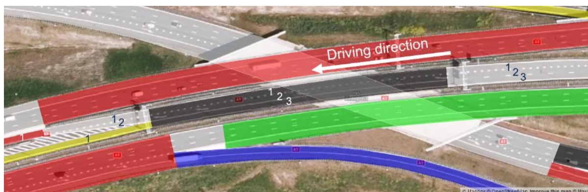
Figure 34: ADASIS-road segments and ADASIS lane numbering for the central crossing of scenario in clause 3.3 (where the motorways crosses each other). (Source: created using https://geojson.io © Mapbox (see: https://www.mapbox.com/about/maps/ ) © Maxar (see: https://www.maxar.com/ ))
