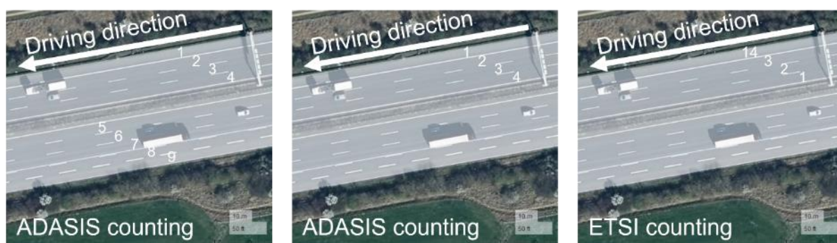
Figure 23: Example of the transformation algorithm, based on an imaginary ego within the segment. The white segment of this figure corresponds to the long blue segment in Figure 20. (Source: created using https://geojson.io © Mapbox (see: https://www.mapbox.com/about/maps/ ) © Maxar (see: https://www.maxar.com/ ))
