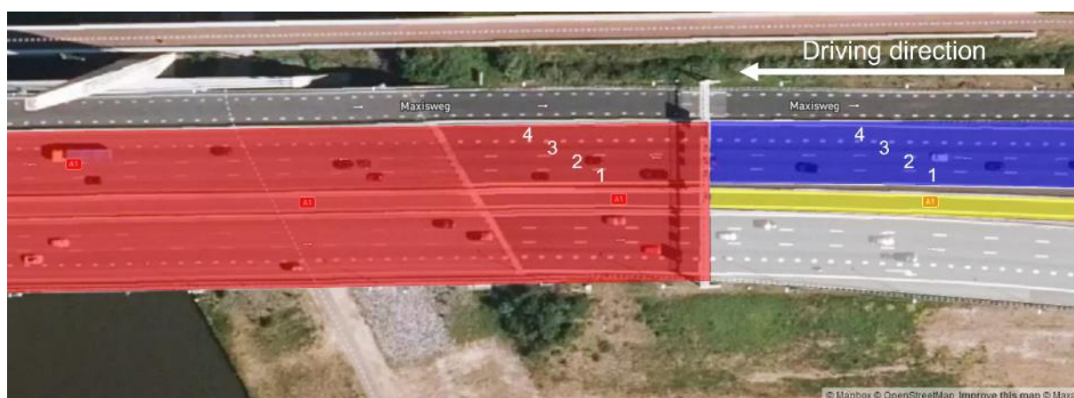
Figure 33: ADASIS-road segments for the 'Muiderbrug' of scenario in clause 3.3 (where the exit lane starts) with the expected ETSI LanePositions. (Source: created using https://geojson.io © Mapbox (see: https://www.mapbox.com/about/maps/ ) © Maxar (see: https://www.maxar.com/ ))
