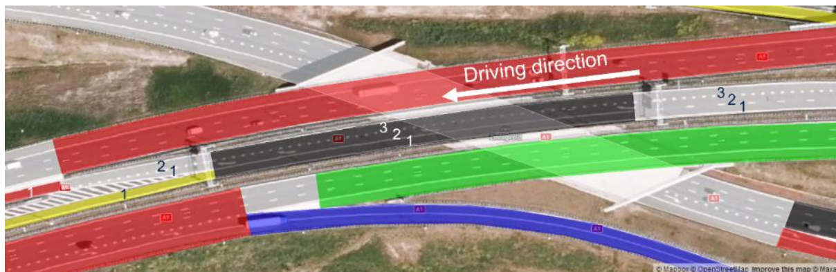
Figure 35: ADASIS-road segments for the central crossing of scenario in clause 3.3 (where the motorways crosses each other) with the expected ETSI LanePositions . (Source: created using https://geojson.io © Mapbox (see: https://www.mapbox.com/about/maps/ ) © Maxar (see: https://www.maxar.com/ ))
