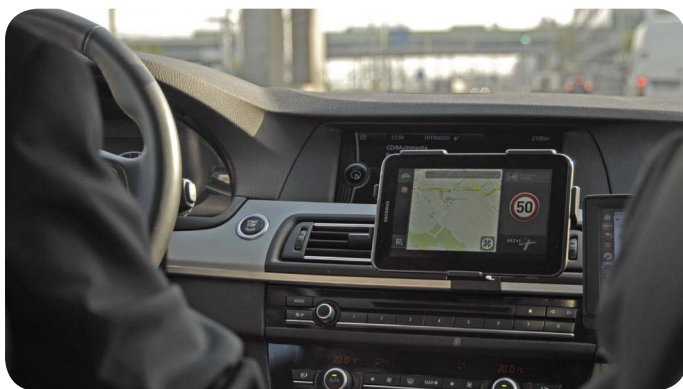
The demonstration route led through the testfeld telematik, the public road network around vienna. The picture shows the in-vehicle signage application informing the driver about current speed limits.
