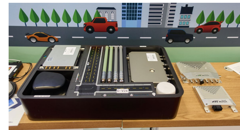
Three generations with V2X communication hardware was presented: DSRC WLANp, C-V2X based on Quectel and 3rd generation based on Qualcomm chipset
