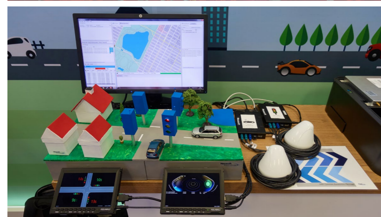
Based on DSRC technology we demonstrated use-cases: Green Light Speed Advisory and Smart Engine Start-Stop function.
