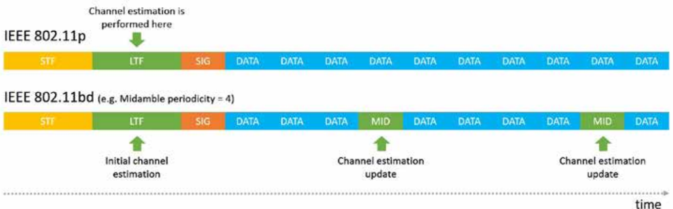
Preamble-based vs midamble-based channel estimation
