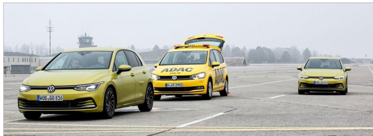
Test scenario: The car with a breakdown warns the following traffic. ADAC C2X Tests with VW Golf 8
